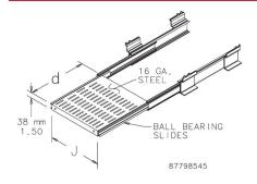
Pull-Out Shelf allows easy access to shelf-mounted devices. Shelf is 1,5 mm steel. The entire assembly is finished with RAL 7035 textured, light-gray polyester powder paint. The shelf mounts to the front surface of front and back 19-in. rack angles.
