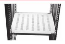
Vented Frame Shelf mounts to the vertical hole pattern on a frame and provides a stationary surface for equipment. The shelf is 1,5 mm steel finished with RAL 7035 textured, gray polyester powder paint.
